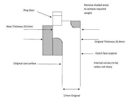
Amount removed will vary depending on fly wheel and cover used F-1600 Area to machine to achieve new proposed min weight
