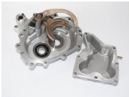
LD200 and MK8/9 genuine Hewland Parts and CNC machined of O ring grooves into Mk8/9 cases
