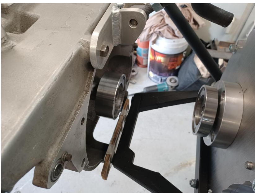
Note curved diagonal and relocated roll-hoop stay
